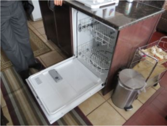
Door spring does not function
